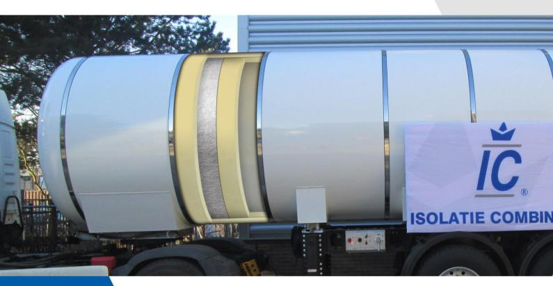
IC offers a high quality cold insulation system for trailers and mobile tanks with this PU (poly urethane) insulation
